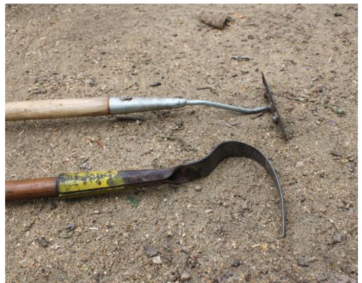
Gung Hoe (top) and Trojan single pronged hoe (bottom). Both are suitable for scuff hoeing.
